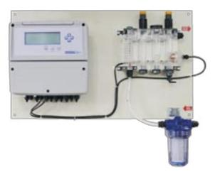
Its universal power supply 100 – 240 Vac 50/60 Hz 20W delivers high technical performance and the **galvanized electrical** and **measuring insulation** ensures reliability.
